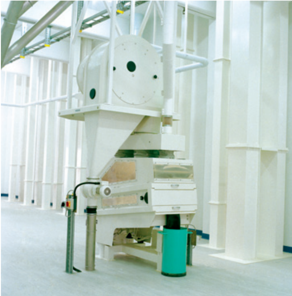
Destoner MTSC. Execution with air-recycling system and two screen decks.
